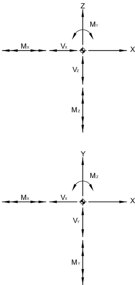
Figure 1: Forces acting on the pile head at any time during seismic event.
