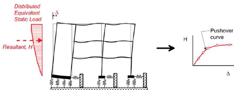
**Figure 1.** Example pushover analysis for Nonlinear Static Procedures (NIST 2012).
