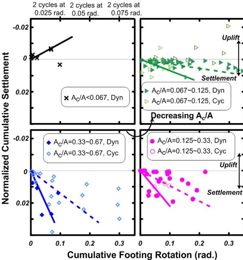
**Figure 10.** Normalized cumulative settlement as a function of cumulative footing rotation for different ranges of  $\rho_{ac}$  (Hakhmaneshi et al. 2012, 2013; Deng and Kutter 2012). Dashed lines represent median relations and solid lines are the envelopes proposed by Deng et al. (2014).
