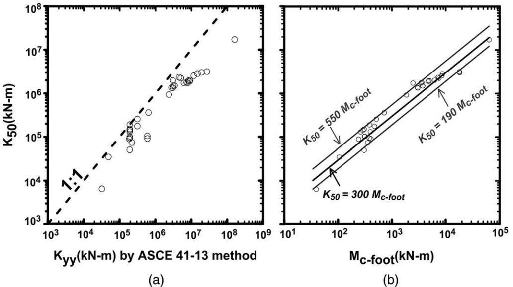
**Figure 12.** (a) Comparison between stiffness computed using FEMA (2000) equations (e.g., Equation 4a) and  $K_{50}$  obtained by fitting experimental data to the trilinear model. (b) Correlation between moment capacity of a rocking footing and  $K_{50}$  (Deng et al. 2014, Hakhmaneshi et al. 2016).
