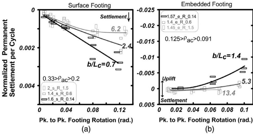
**Figure 9.** Normalized residual settlement per cycle of rotation for rectangular footings in dry sand. (a) Surface footings with  $\rho_{ac} \approx 0.25$  to  $0.35$ . (b) Embedded footings with  $\rho_{ac} \approx 0.1$  (Hakhamaneshi et al. 2014).
