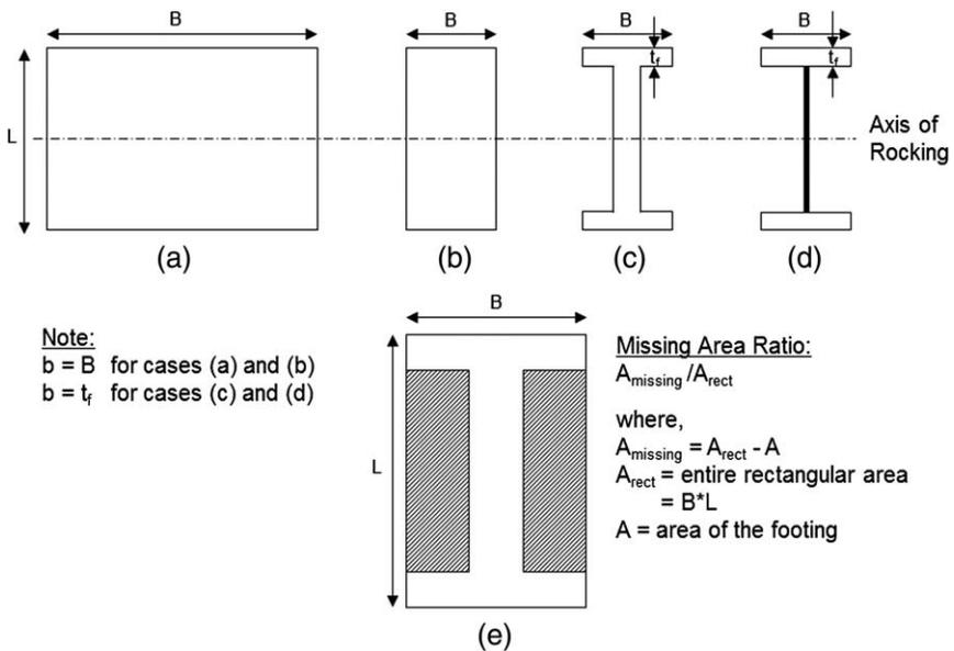
**Figure 5.** Characterization of footing shape.
