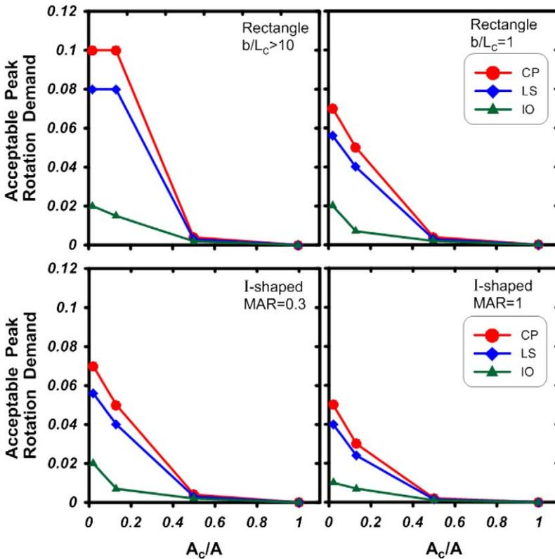
Figure 11. Acceptance criteria for peak rotation demand on rocking foundations.
