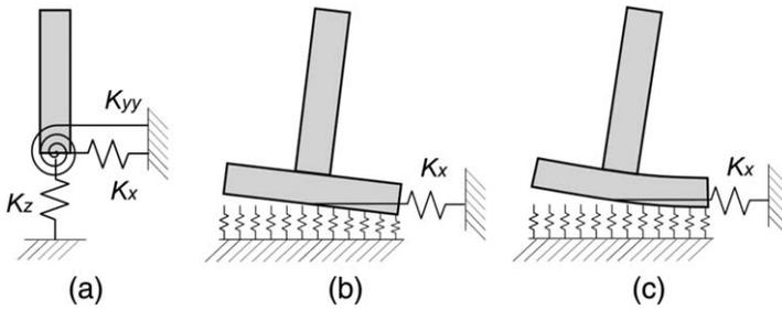
**Figure 2.** Methods for modeling rocking foundations in ASCE 41-13. (a) Method 1 using uncoupled springs, (b) Method 2 using nonlinear sub-grade reaction springs, and (c) Method 3 for cases where, the footing is flexible compared to the soil.
