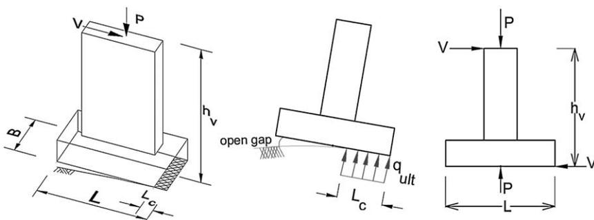
**Figure 3.** Footing shape parameters for rectangular and I-shaped rocking footings.
