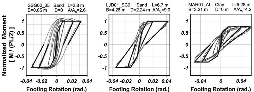
Figure 6. Rotation to mobilize capacity from ASCE 41-13 and experiments.
