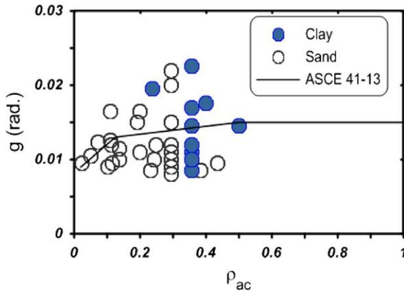
**Figure 7.** Observed relationship between footing rotation to mobilize moment capacity and the inverse of  $\rho_{ac}$  for rectangular footings in model tests.
