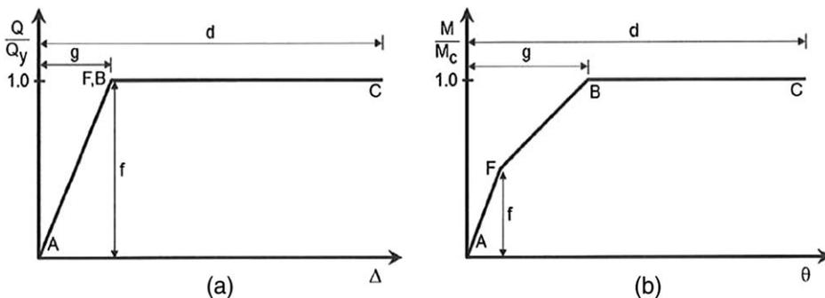
**Figure 4.** Load-deformation behavior for shallow foundations using Method 1 (uncoupled foundation springs) with a (a) bilinear relation for axial loading and shear loading, and (b) trilinear model for moment-rotation behavior.
