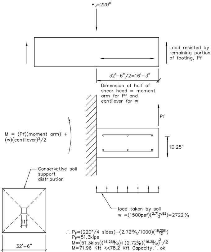
Figure 5: Shear head flexure check.
