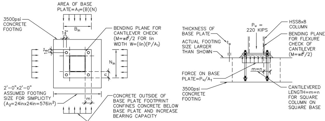
Figure 1: Bearing plate check.
