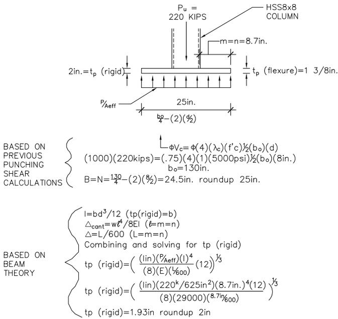
Figure 3: Rigid base plate calculation.
