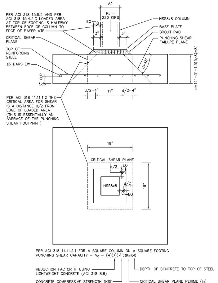
Figure 2: Punching shear.
