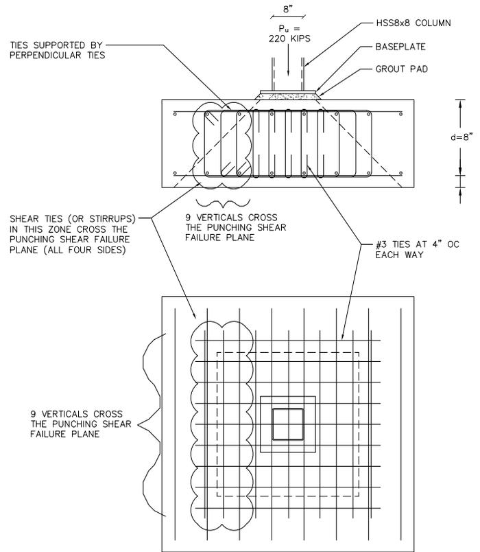
Figure 4: Shear head reinforcement.
