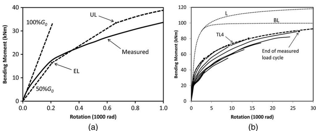
**Figure 7.** Comparison of predicted and observed rotations from tests of narrow footings on silty clay: (a) close up of first cycle, (b) all nine cycles of monotonic loading. Field test data from Algje (2011).
