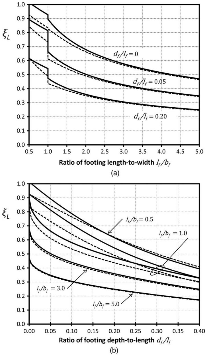
**Figure 1.** Non-dimensional parameter accounting for footing geometry on initial rotational stiffness.
