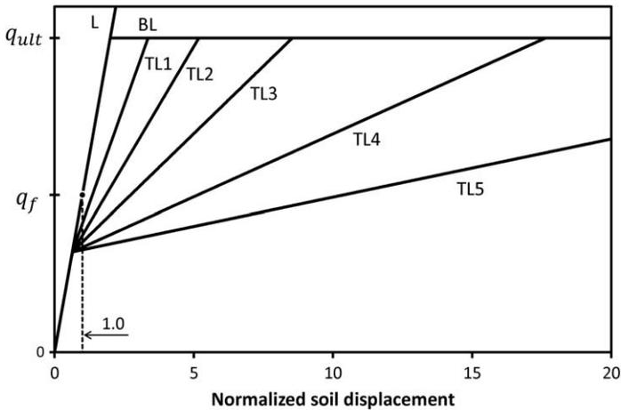
**Figure 2.** Relationship between bearing stress (vertical axis) and normalized soil displacement defined by different Winkler springs: L = linear, BL = bilinear, TL = trilinear.
