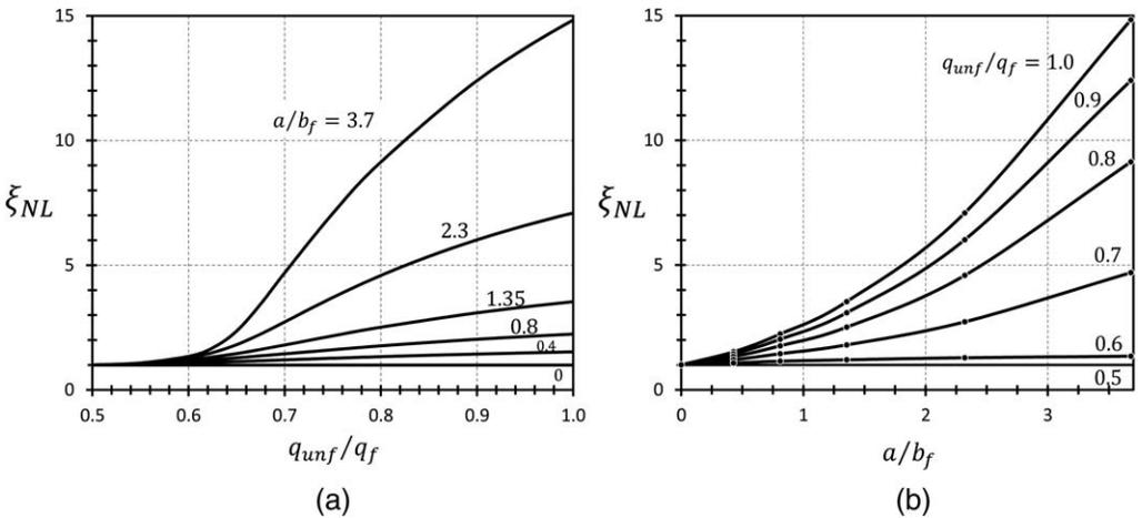
**Figure 9.** Non-dimensional parameter accounting for increased footing rotation due to nonlinearity of soil as a function of magnitude and length of required uniform bearing stress.
