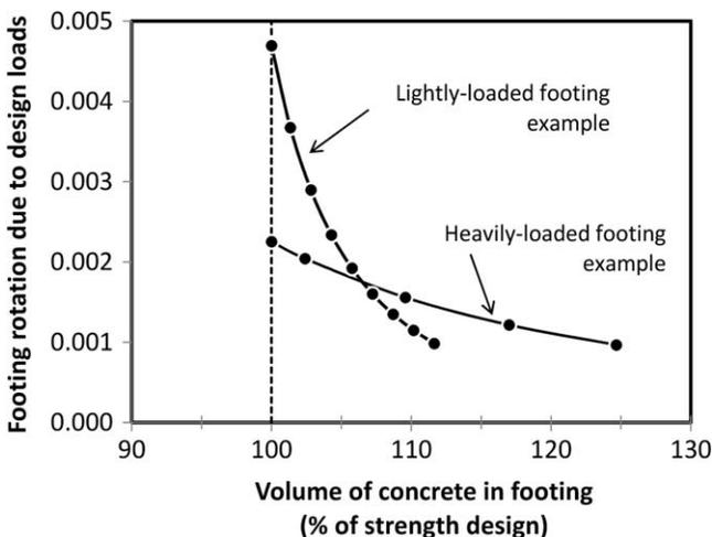
**Figure 10.** Results of two footing design examples showing the reduction of footing rotation due to increased footing size relative to the minimum strength requirement for a lightly loaded rectangular footing and a heavily loaded square footing.
