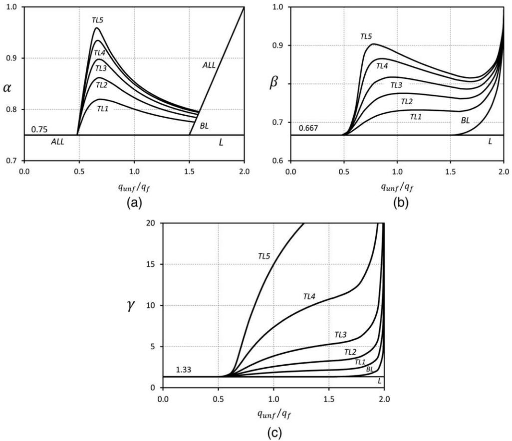
**Figure 4.** Parameters defining the statically equivalent uniform bearing stress distribution for different Winkler springs: (a)  $\alpha$  = ratio of uniform bearing stress to maximum actual bearing stress, (b)  $\beta$  = ratio of uniform bearing stress length to actual bearing stress length, (c)  $\gamma$  = ratio of maximum soil displacement to displacement of linear soil subjected to uniform bearing stress.
