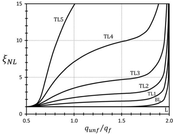
**Figure 5.** Non-dimensional parameter accounting for increased rotations due to nonlinearity of soil resulting from different Winkler springs.
