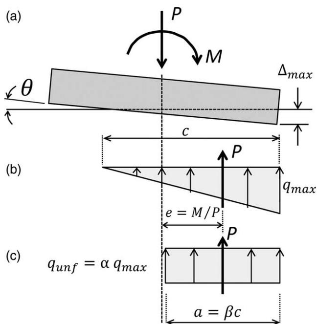
**Figure 3.** Statically equivalent uniform bearing stress: (a) rotating footing, (b) resulting bearing stress distribution from linear soil, (c) uniform bearing stress with statically equivalent resultant.
