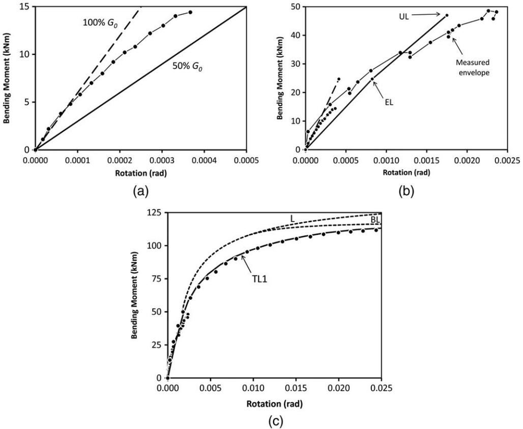
**Figure 6.** Comparison of predicted and observed rotations from tests of square footings on sand: (a) envelope of small-amplitude force-controlled cycles, (b) envelope of earthquake time history, (c) envelope of increasing cycles until overturning capacity. Laboratory data from Negro et al. (1998).
