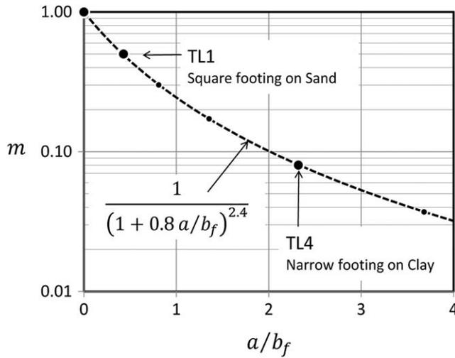
**Figure 8.** Proposed relationship between secondary slope of trilinear Winkler springs  $m$  and ratio of uniform bearing stress length to footing width  $a/b_f$ .
