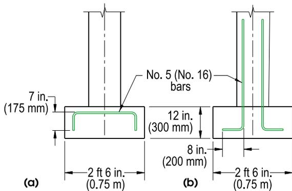
**Fig. 3:** Because the “A or G” dimension is 10 in. (250 mm) for a No. 5 (No. 16) bar (refer to Fig. 4), the restricted depth provided in this footing will necessitate rotation of the 90-degree hook extensions on: (a) the footing bars; and (b) the column dowels
