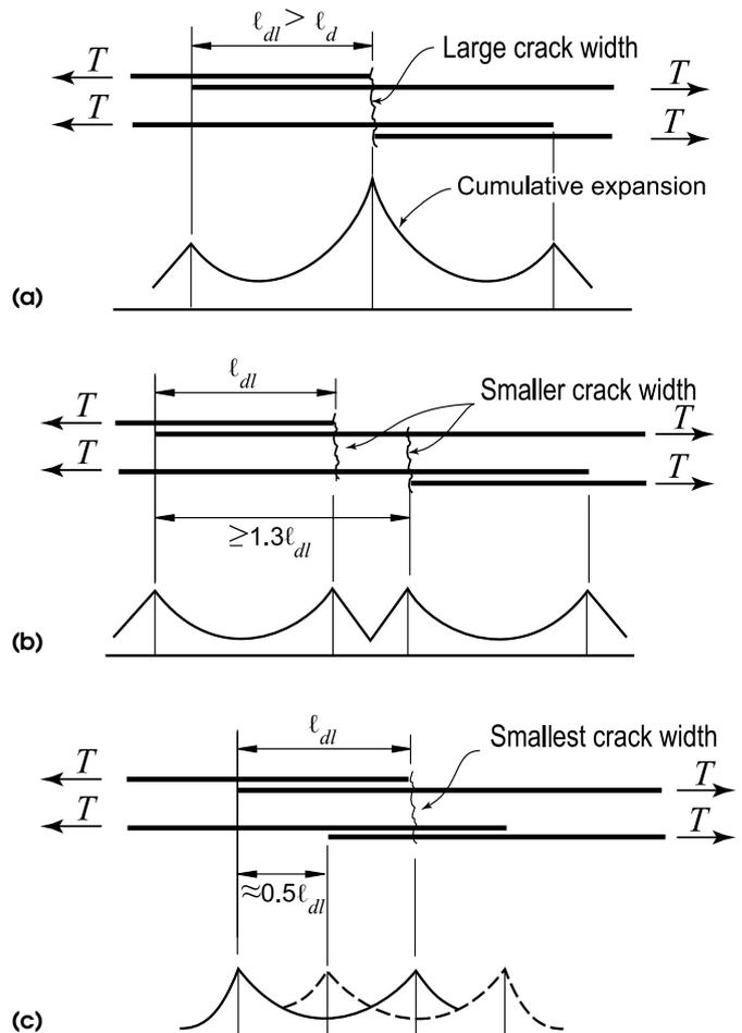
**Fig. 6:** Crack widths are functions of splice locations: (a) superimposed effects can be adverse, resulting in large crack width even when lap length  $\ell_{dl}$  exceeds tension development length  $\ell_d$ ; (b) avoiding superposition reduces crack width; and (c) low superposition results in smallest crack width (based on Reference 7)
