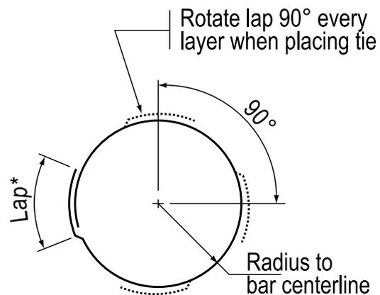
\*Class B splice modified for top bar and coating
